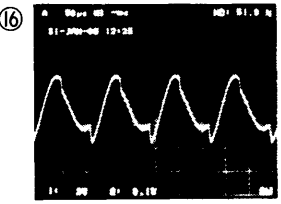
IC 303 Pin ⑪ 1/2 fH Resonance (2V/50µsec)
